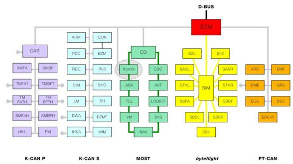
The communication with control units in the chassis, power train and body areas is via the K-CAN System.
